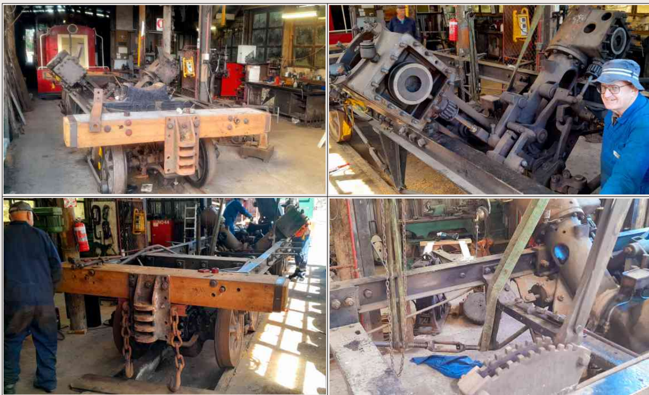
Above: A big Heisler work weekend recently – headstocks, cylinders, cab measure, etc. (JS)
