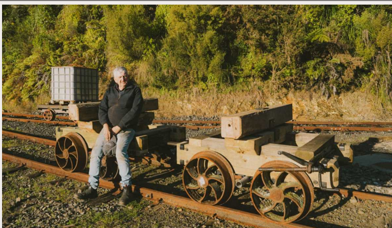
Above: The log bogies: new timber with original steel fittings (Bruce McL, JS)
