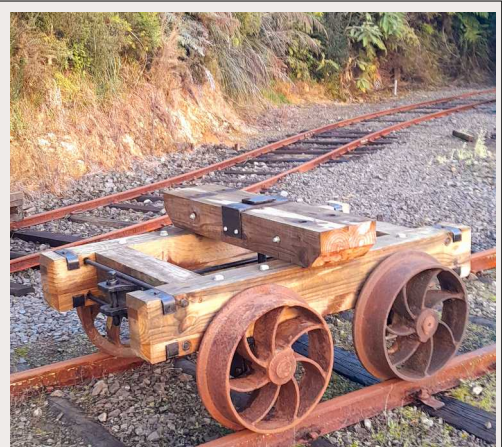
Above: The log bogies: new timber with original steel fittings (Bruce McL, JS)
